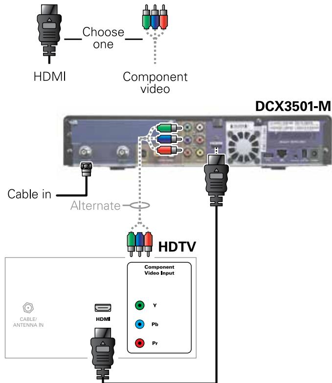
**Note:** Because HDMI provides both video and audio output, no additional audio connections to the TV are required.
