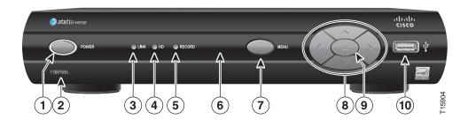
**1 Power**Turns the receiver on or places it in standby. To restart the receiver, press and hold the POWER button for 10 seconds. The LED is green
