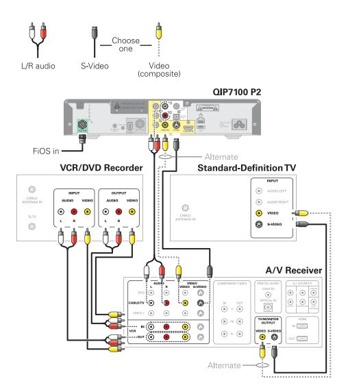
Note: Because some entertainment equipment cannot simultaneously support composite video and S-Video, never simultaneously connect both video inputs.
